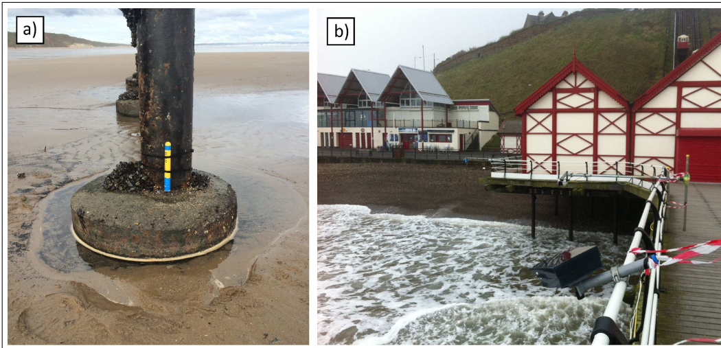
Figure 2.10: Photographs of one in situ and one remote sensing instruments: a) example of pressure transducer deployed close to the sea bed in the macrotidal environment of Saltburn; and b) example of camera deployment for coastal monitoring (Photos taken by the author during the field experiment presented in Chapter 5).
